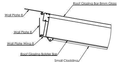
Roof Glazing Bar & Sheet Section
