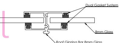
Eaves Beam, Roof Glazing Bolster Bar & Post Section
